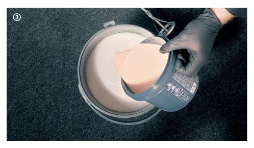
Tip: in order to improve the visibility of the processing, Wallcrete in paste form can be coloured by adding a few drops of Decor of the same shade as the final colour.
