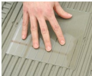
Wettability test: a simple pressure is enough to obtain full-bedding under the tile
