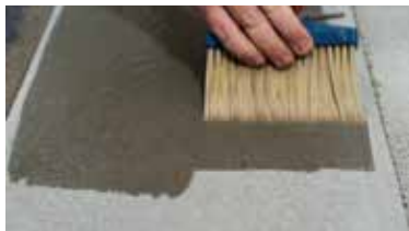
CONCRETE checking absorption
